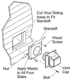
Figure 24 - Installing Vinyl Siding Standoff
